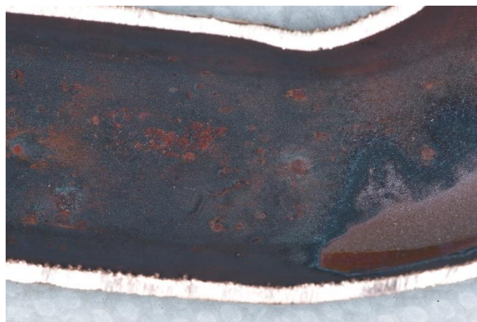
Figure 4 – Scale on ID of Return Bend
