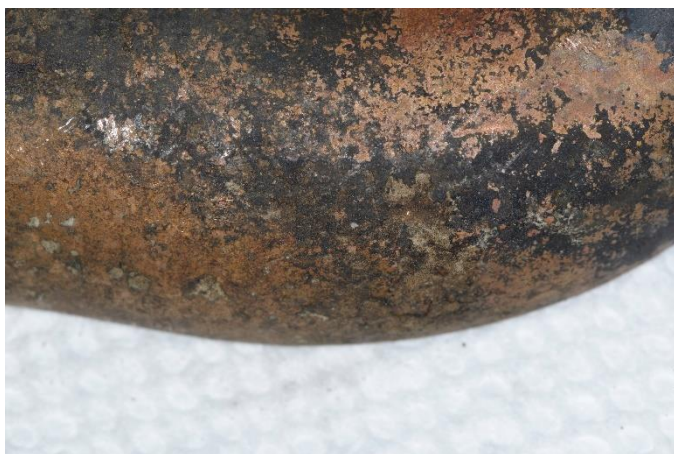
Figure 3 – Scale on OD of Return Bend
