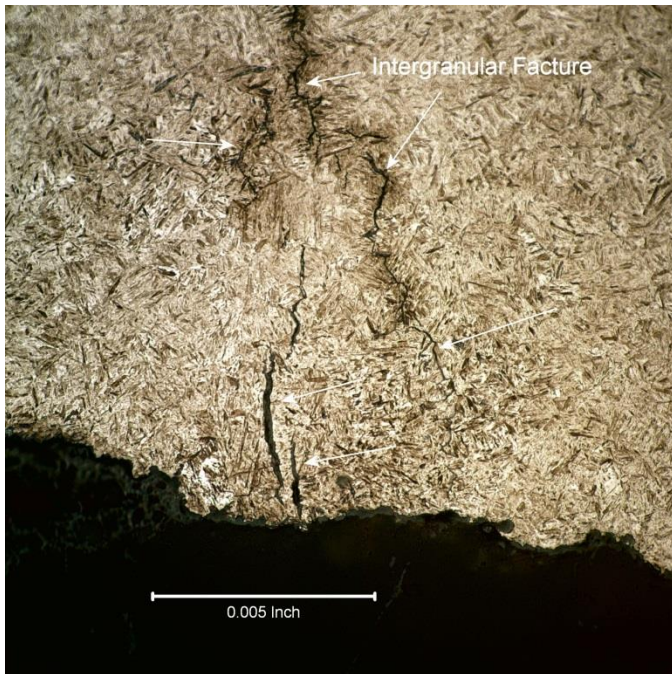
Figure 3 – 400X Intergranular Fracture, Sample 2
