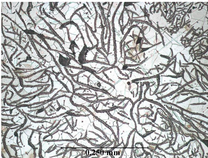
Figure 7 – 200X Ferritic Gray Cast Iron – Flange Area of Fracture
