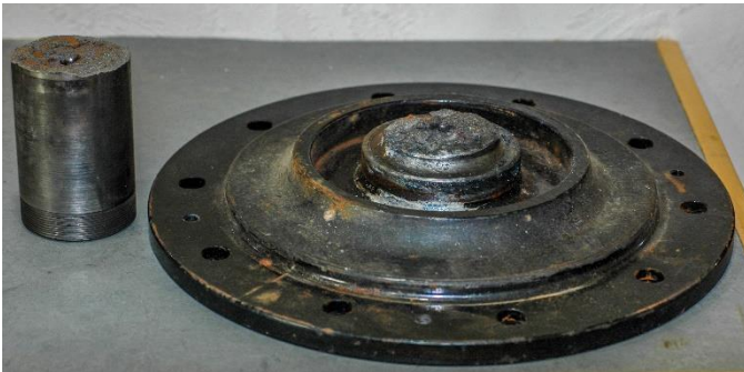
Figure 1 – Broken Casting as Received from Client
