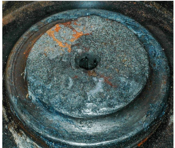
Figure 2 – Hub Flange Fracture
