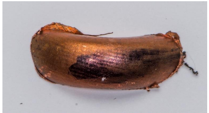
Figure 2 – Leak Indications on Outside of Hairpin
