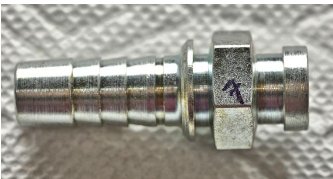
Figure 1 – Zinc Plated Steel after Five Months in Storage
