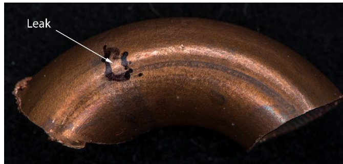
Figure 3 – Leak Location O.D. of Hairpin
