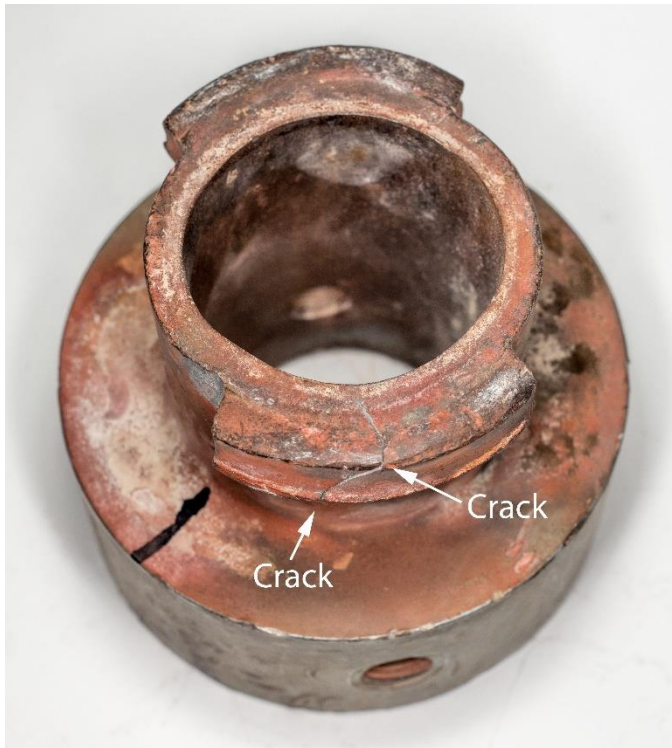
Figure 1 – Crack in Lug, Locking Clamp 1
