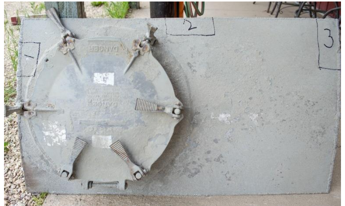
Figure 3 – Panel Blown from Top of Trailer
