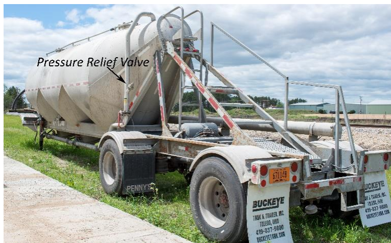
Figure 1 – Trailer and Pressure Relief Valve
