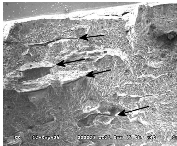
Figure 6 – 40X Fissile Fracture
