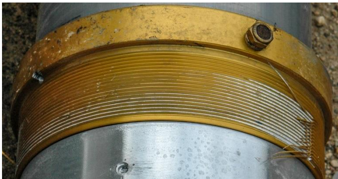
Figure 3 – Sheared Threads on Cylinder End Cap
