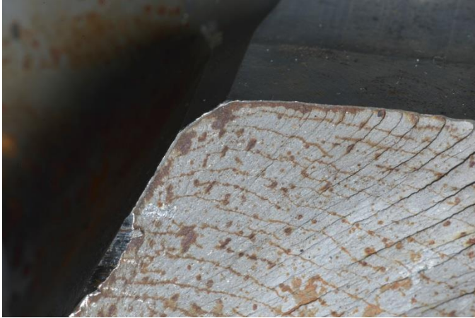
Figure 3 – Flat Fracture and Very Small Shear Lip
