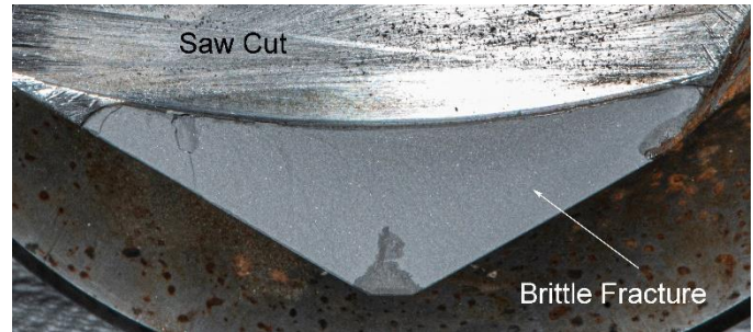
Figure 4 – Saw Cut and Brittle Fracture
