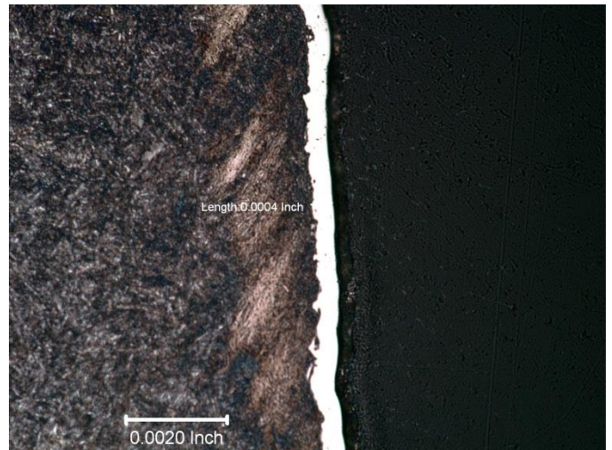
Figure 6 – 400X Nickel Plating on Pawl Surface
