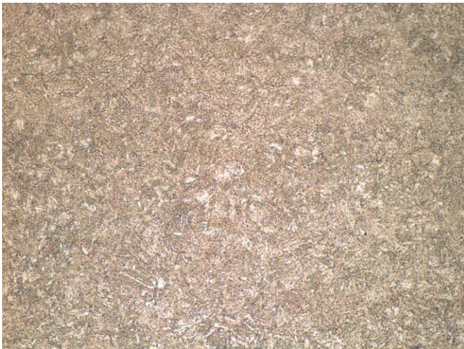
Figure 5 – 400X Tempered Martensite Microstructure, Bolt 2
