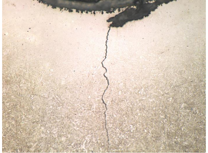
Figure 8 – 400X Intergranular Cracking, Thread Root, Bolt 2
