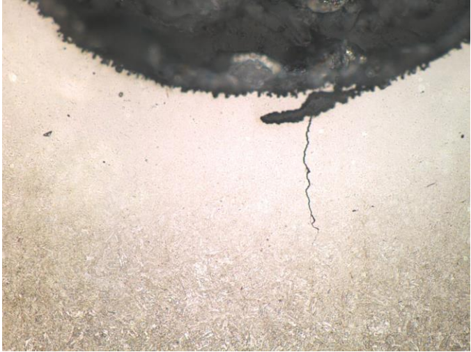
Figure 7 – 400X Intergranular Cracking, Thread Root, Bolt 2
