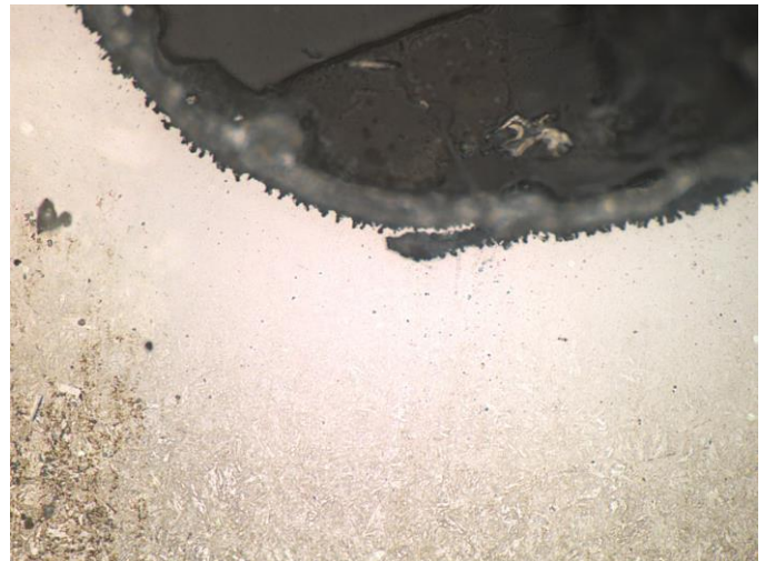
Figure 6 – 400X Pitting Corrosion Thread Root, Bolt 2
